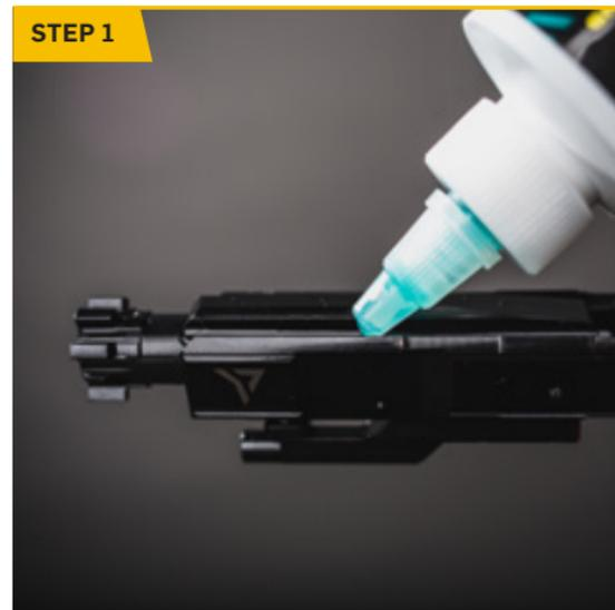
*The bolt carrier body and cam pin, especially along the runners on the bottom of the carrier and the bosses on the rear, should be lubricated. Place two drops of lubrication into the cam pin slot.*
