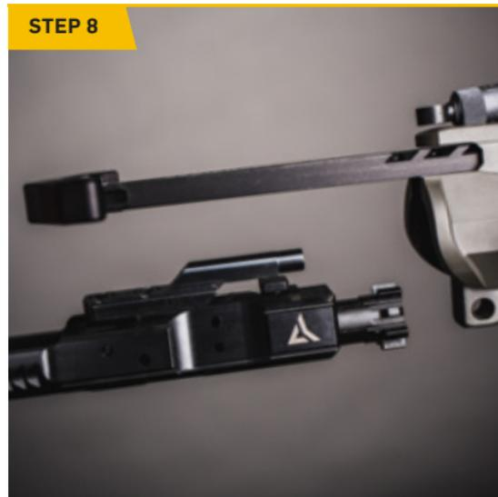
*Remove the bolt carrier group from the upper receiver.*
