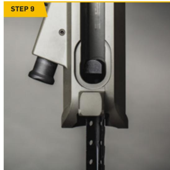
*Pull the charging handle fully towards the rear. Remove the charging handle by moving it so that the expanded end of the charging handle passes through the cut-out in the guide track of the upper receiver.*
