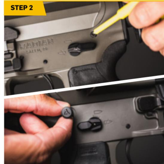
Make sure the bolt carrier group is in the forward seated position. From the left-hand side, press in the rear takedown pin. From the right-hand side, pull the rear takedown pin to the right until it stops.
