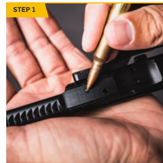
*With a suitable punch or the tip of a cartridge, push the firing pin retainer in from the **right-side**, then pull it out from the **left-side**. Do not twist the retainer during removal.*
