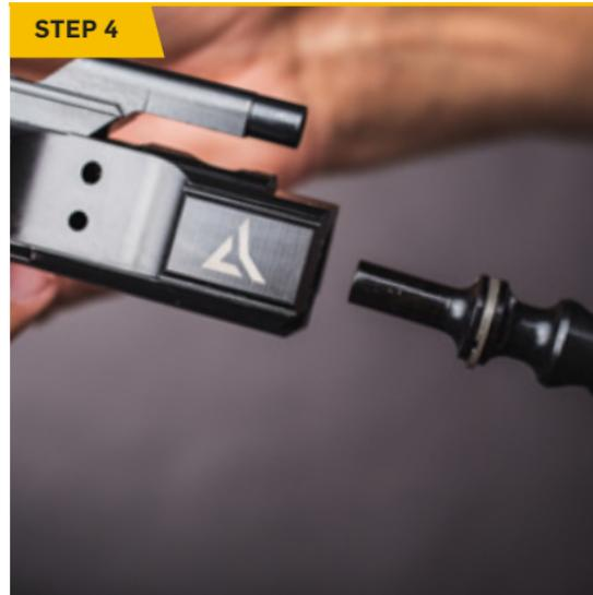
*Remove the bolt from the front of the bolt carrier.*
